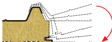
Isofire Roof Fono panel assembly system
